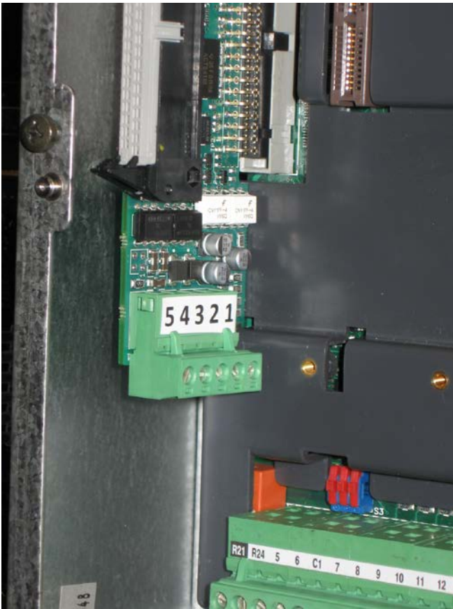
Figure 5. Terminal numbers on XSC
